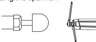
Make the die grinder run in idle for at least a minute with the grinding point correctly assembled, the grinding point should be immediately replaced if there is the vibration.
