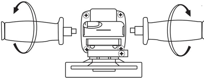
**■ INSTALLING OR REMOVING WHEEL GUARD**
